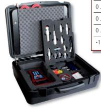
Measuring set 4010A-ppTQ with sensors for pressure, temperature and volume flow rate, Minimess® connectors and accessories; the image shows optional components, like additional sensors, Patrick the particle counter and a MultiXtend module.
